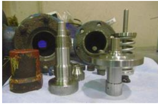
Plate 2 Picture of Cleaned PRV parts
