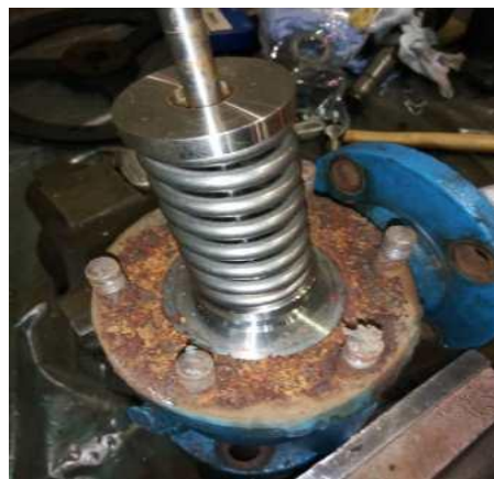
Plate 1: Picture Depicting Occurrence of Corrosion
